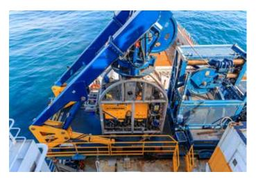
Deep-sea submersibles are connected to the surface operating ships via cables that carry power and communications. The single umbilical cables will contain several individual cables held within an outer sheath.
