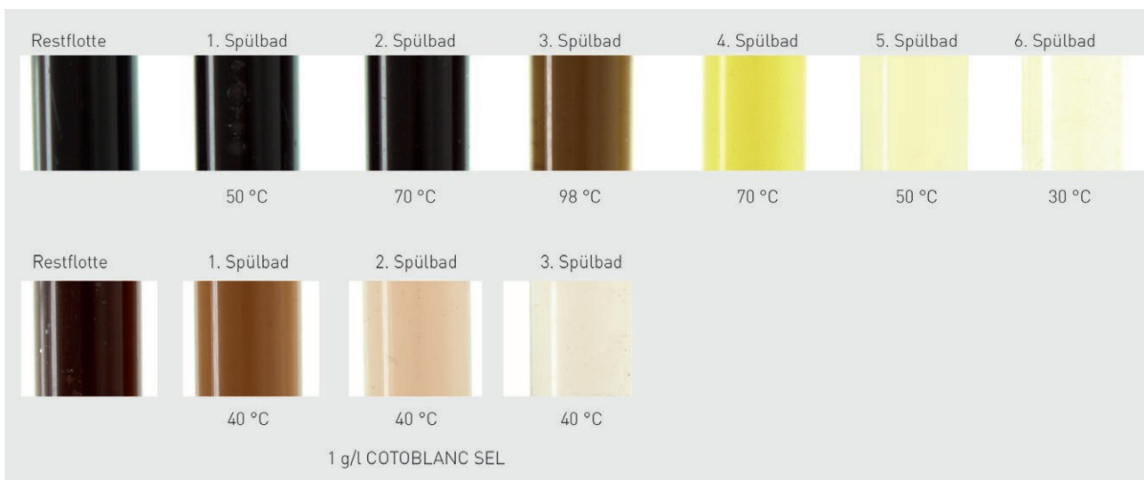
Fig. 2: Comparison of the rinsing baths in the reactive dyeing process (top: commodities / bottom: process at 40 °C using BEZAKTIV GO and COTOBLANC SEL).
